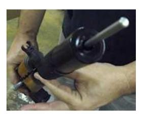
Now place the suppressor into the jig positioning the gun horizontally so that you will cut the pin hole on bottom side of suppressor. Use a wood block or something to support the gun and keep it level.
