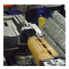
Use a fairly high spindle speed (1700 RPM) and "peck" drill cutting short depths and pulling all the way out multiple times. Blowing shavings away and/or applying coolant (water) each time the drill is pulled out will help keep it sharp.
