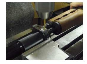
Check the depth of your hole to make sure that it is deep enough that the pin will go below flush when driven in. The pins that we supply are intentionally oversize for a tight fit. It will be helpful to sand or file the outside of the pin slightly to the point that it goes in about half way without hammering. Also, one side is intentionally smaller than the other so start that side into the hole first.
