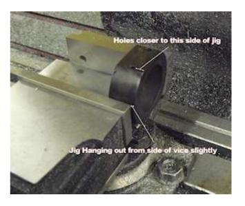
Line up the 5/32 drill so that it is centered with the small hole in jig. Once it is very close to center turn the drill on and run it in and out of the hole looking carefully from side and front and adjust to minimize deflection.
