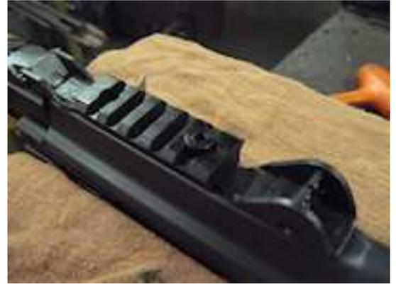
Remove the rail and bushing. Then drill the one hole through using the previously drilled spot as a guide.
