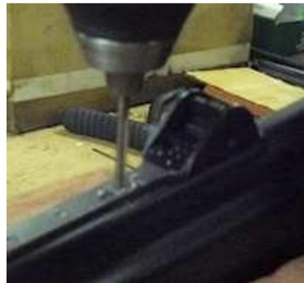
Once this hole is cut, go ahead and thread it with the supplied tap. A good tap handle and cutting fluid, such as Tap Magic ®, are very helpful for this step. Make sure to keep the tap straight in line with the drilled hole and go slow, applying firm downward pressure while cutting, and occasionally unscrew it back a little ways to clear chips.
