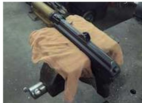
Place the rail over the top cover hinge arm between the hinge and rear sight block.
