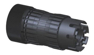
For standard AK, eight detent cuts are available for close attachment to muzzle. It is trepanned for weight reduction and outer diameter slots provide access to detent for installation/removal.
