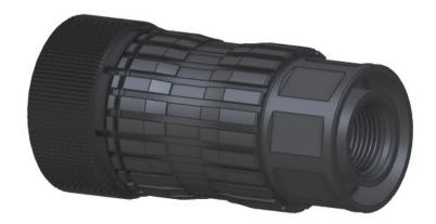
For 5/8-24, the detent notches are replaced with wrench flats to allow tightening to a crush washer or jam nut. Rear is trepanned for weight reduction, while the larger diameter provides better look on the gun.
