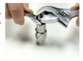
The pilot should now have minimal play from front to back but still be able to spin freely inside the cutter.
