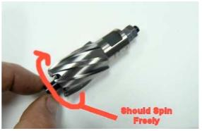
3) Line up the 2 set screws in the shank adapter with the 2 flats on the 3/4" annular cutter shank.
