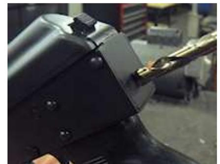
Once the hole is drilled you may want to deburr the inside of the receiver and cold blue the bare metal for rust prevention. The buttstock nut should be placed on the inside of the receiver with large radiused edges facing the rear and on the left and right sides (rather than top and bottom).
