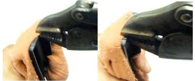
If you have to bend this surface substantially, this can possibly bow the metal just below the hole where the recoil spring locks in. This may not be visibly apparent but is probably the case if the top cover lowers all the way down into closed position and the recoil spring still does not completely lock in. To remedy this, we suggest that you take an adjustable wrench and bend it back down slightly as shown.
