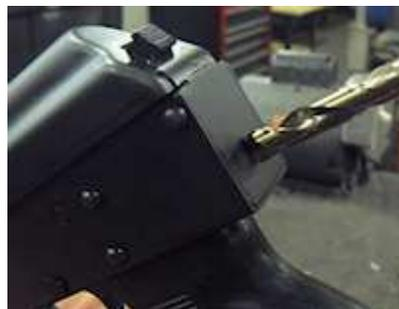
Deburr the hole inside and out as well as you can. Use a cold blue solution to make the machined surface rust resistant if desired.
