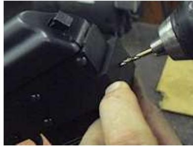
Drill the small hole at a fairly high speed (about 1500 RPM)
