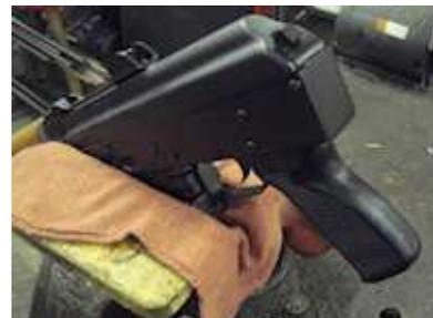
Place the locating jig on the back of the receiver, using the milled steps to locate it from the 2 sides and lower receiver surface
