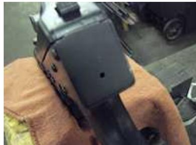
Using the small hole as a guide, drill through with 3/8 drill at a slow speed (about 700 RPM)
