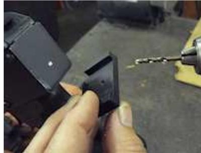
Drill the rest of the way through without the jig in place
